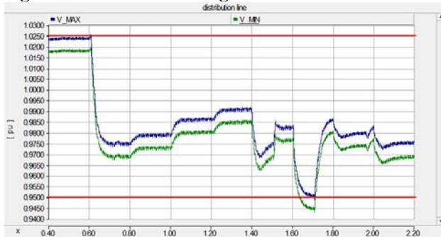
**Fig 12. Simulation of Voltage Control of LDC Method2**
