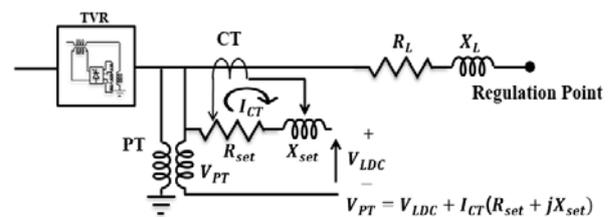
Fig 5. Voltage regulation method by LDC
