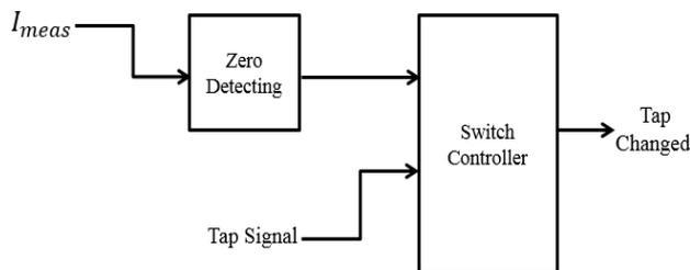
Fig 3. Tab Switch Controller
