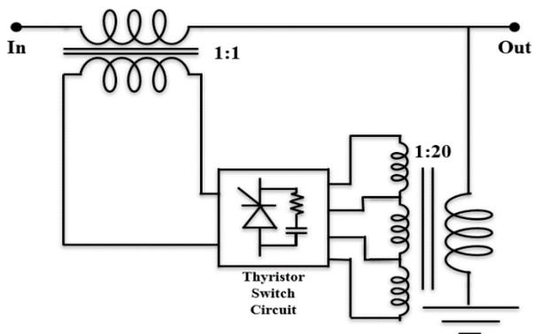
Fig. 2. Single-phase TVR circuit
