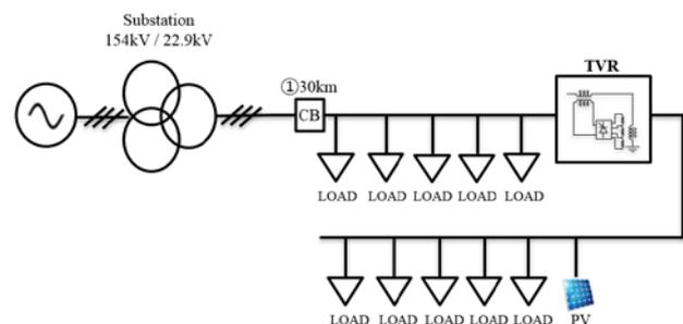
Fig 1. The high-voltage distribution system modeling
