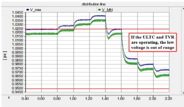
**Fig 10. Simulation of operation with distribution line without voltage control of TVR**
