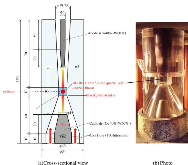
Fig.3. Gas flow nozzle for confinement of decaying arc.
