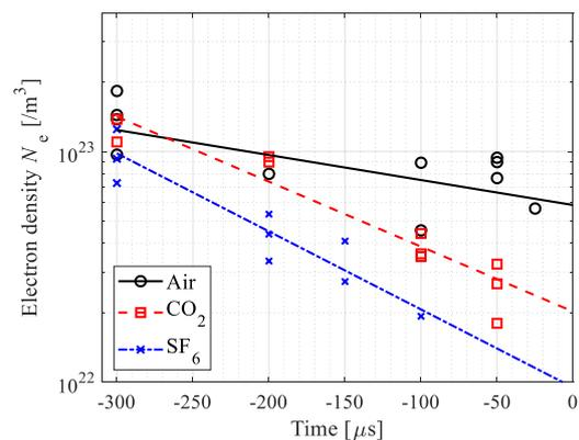
Fig. 7. Time dependence of electron density in nozzle throat under air, CO<sub>2</sub> and SF<sub>6</sub> gas blasting.
