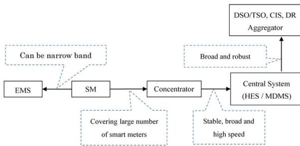
Fig. 1: Typical architecture of smart meter system
