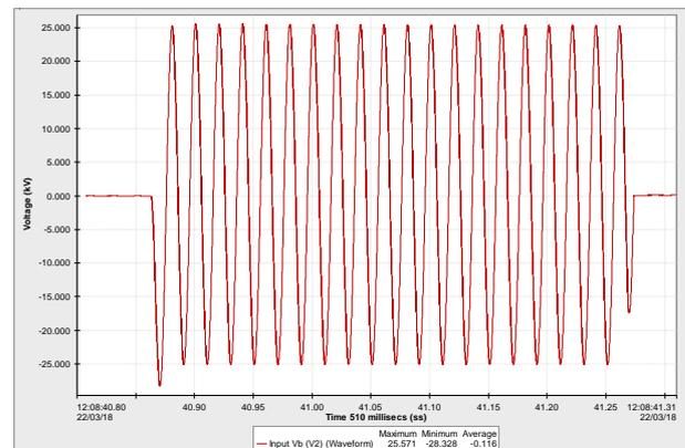
**Figure 6.** Measured earth potential rise (EPR) for Test A.
