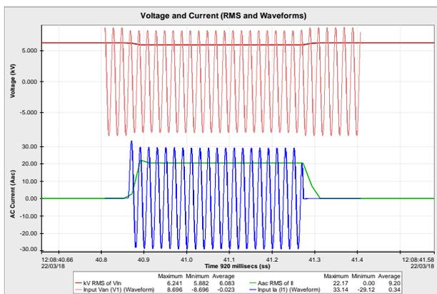
**Figure 3.** Voltage and current waveforms and RMS results for Test A.
