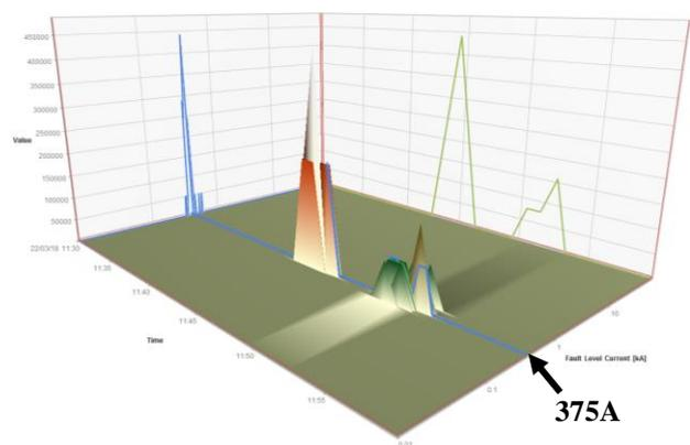
**Figure 5.** Plot of all significant events with a weighted average fault level as the blue line.
