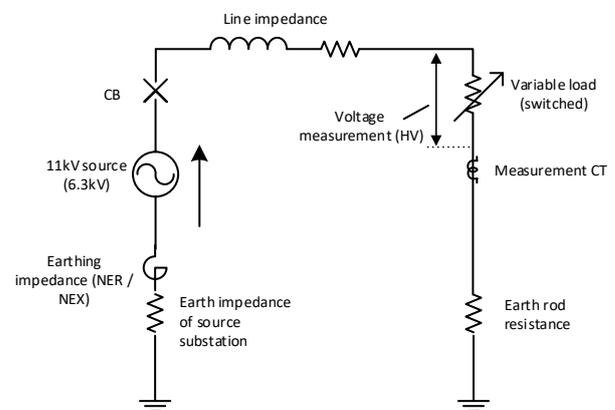
**Figure 2.** Equivalent circuit for the test arrangement.
