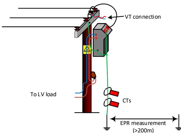
**Figure 1.** Illustration of the measurement connections.
