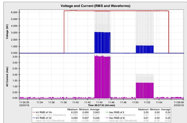
**Figure 4.** Voltage and current waveforms and RMS results for Test B.
