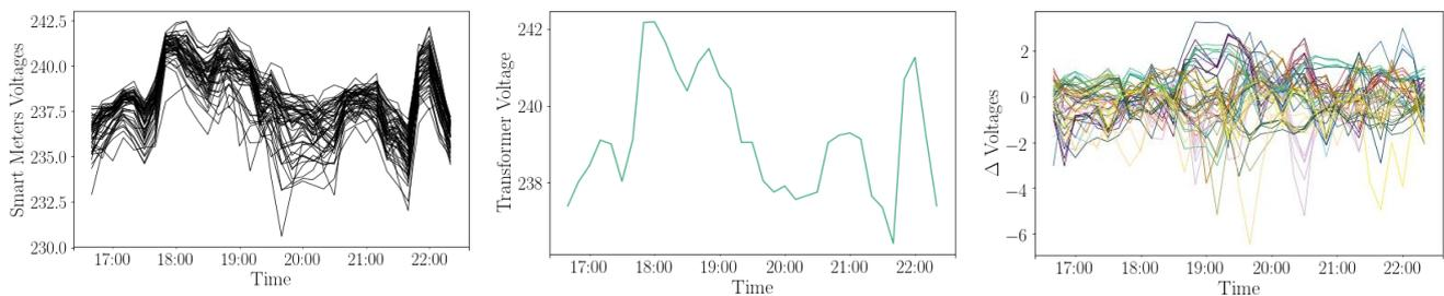
Figure 3: Pre-processing of the voltage data - Removal of medium voltage influence – Example for an identified substation
