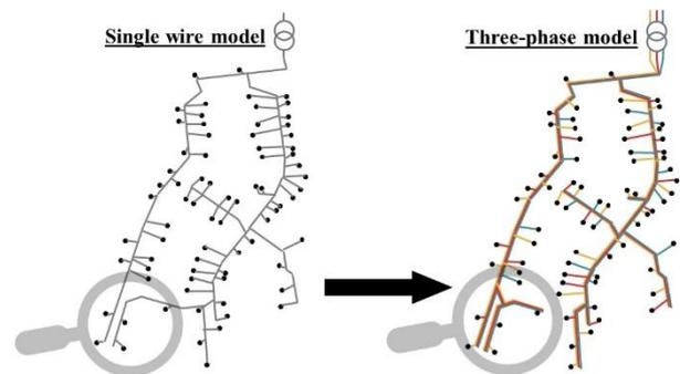
Figure 1: GIS Upgraded: Topology correction & phase connectivity addition
