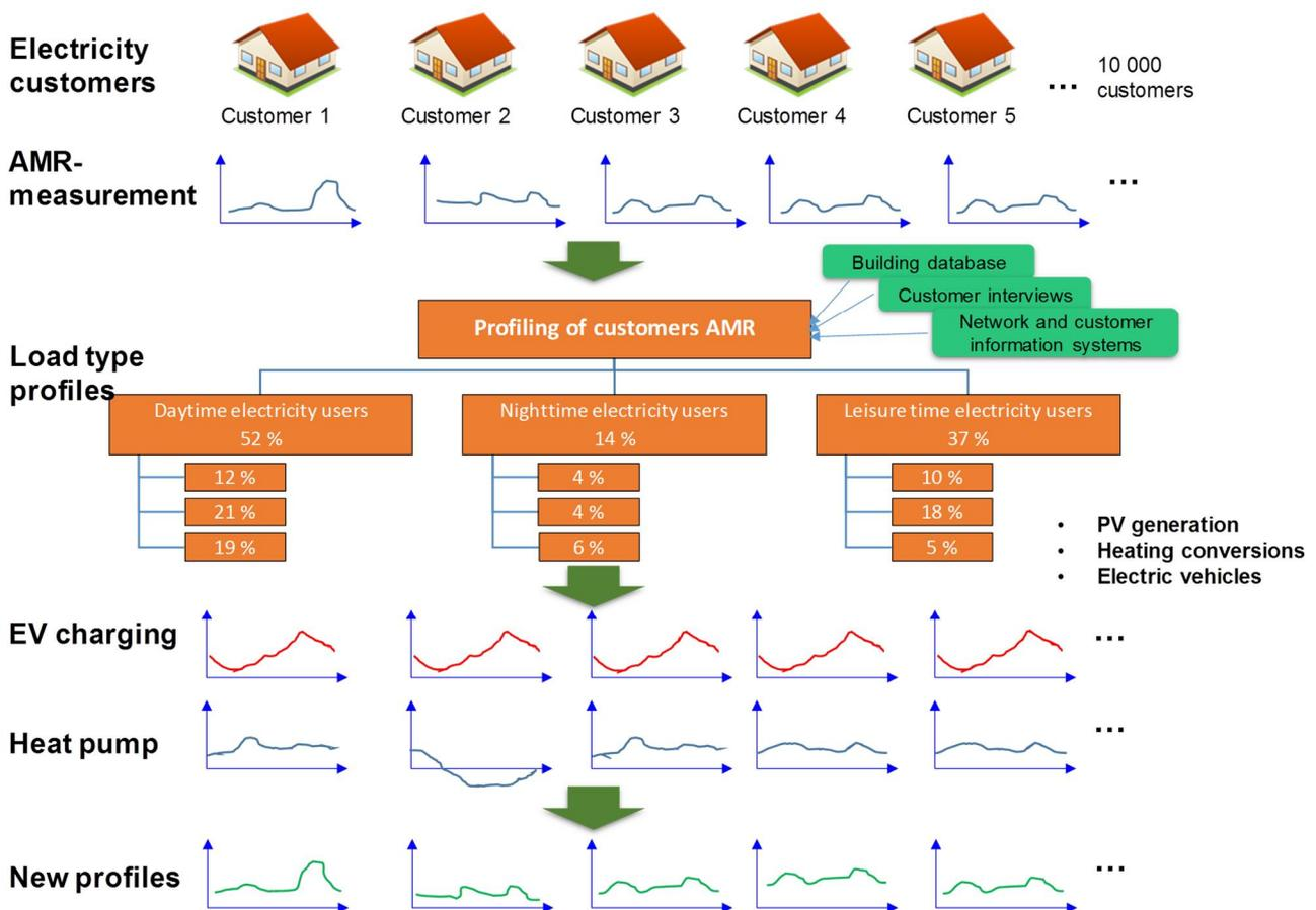
Figure 1. An electricity customer future load profile estimation process.
