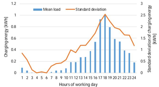
Figure 5. Electric vehicle charging curve (summertime). The energy capacity of the EV battery is 30 kWh and the charging power is 10 kW [6].
