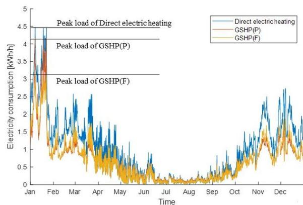
Figure 4. Annual electricity-based heating loads for households with different main heating systems (direct electric heating, full load capacity GSHP, partial load capacity GSHP). The curves are generated from the data of the year 2016 from 10 000 electricity consumption places [4].
