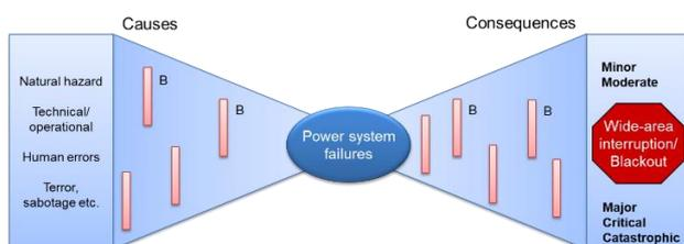
**Figure 1** Bow-tie model for power system failures [3]
