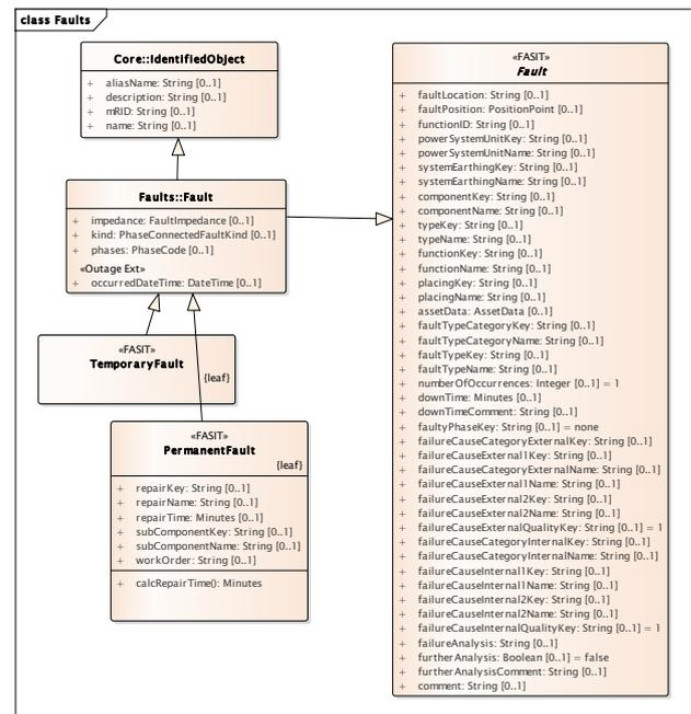
Figure 4 Combination of standard CIM classes and specialized FASIT classes
