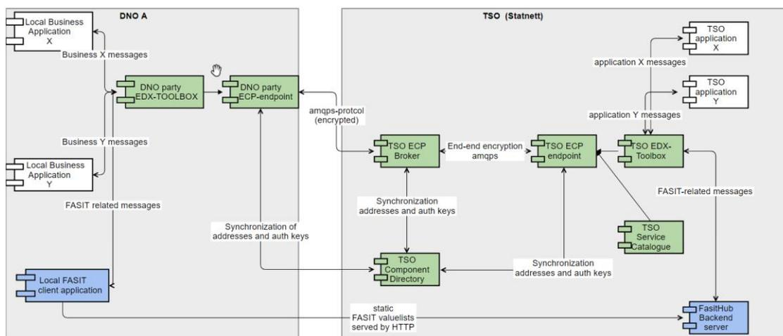
**Figure 9** Example of MADES network and connected business applications
