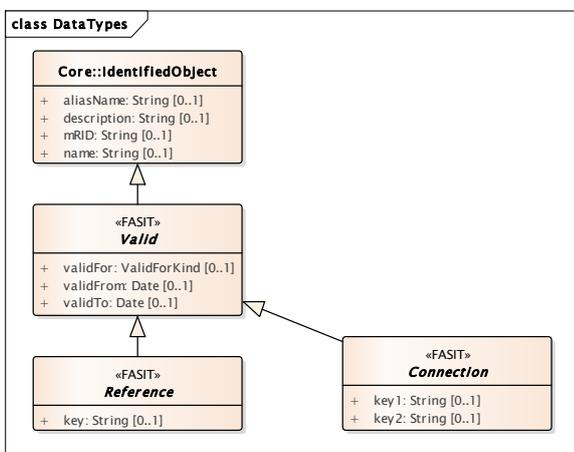
Figure 3 Example of inheritance in FASIT
