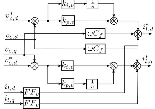
Figure 3: Voltage controller
