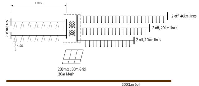
Figure 5-1: 400/110kV underground cable network case
