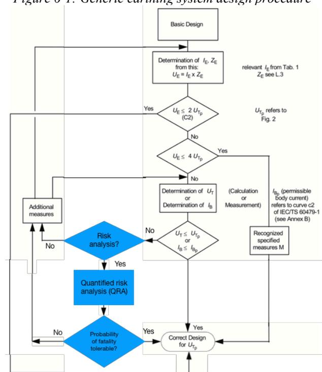
Figure 6-2: EN50522 design process revised to incorporate QRA
