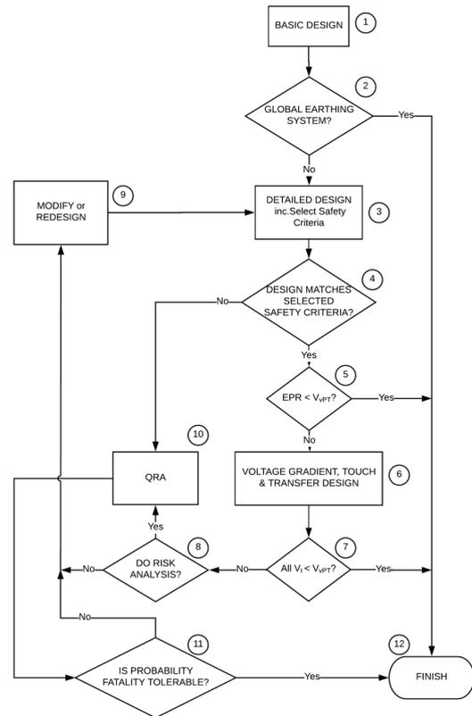
Figure 6-1: Generic earthing system design procedure
