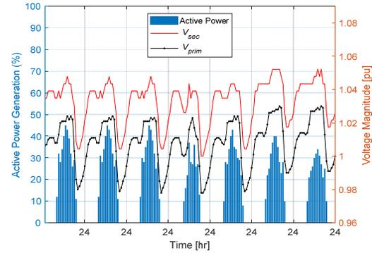
Figure 9. Active power and voltage levels with APC method.
