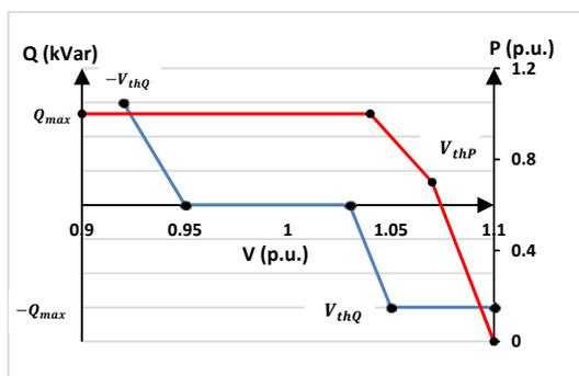
Figure 1. Sequential RPA-APC control of PV inverters.
