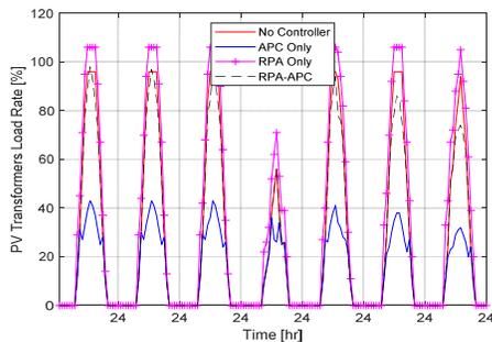
Figure 11. Comparison of load rate of transformer connecting to PV.
