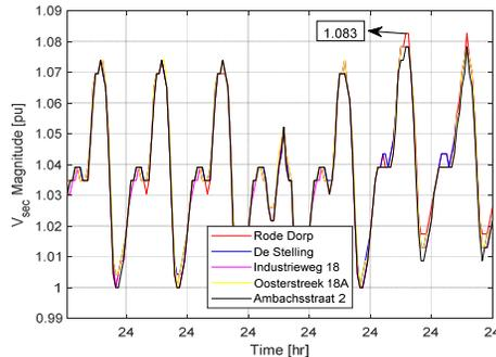
Figure 8. Secondary voltage levels of five feeders directly connected to NW substation.
