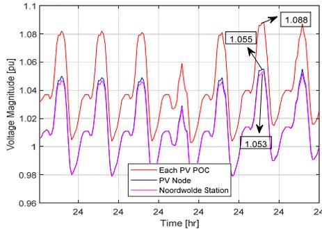
Figure 7. Voltage levels at POC, PV Node, and NW substation.
