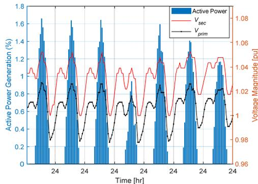
Figure 10. Active power and voltage levels with RPA-APC.
