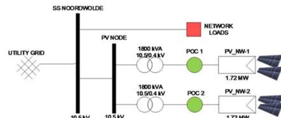
Figure 2. New PV systems connected to NW substation.
