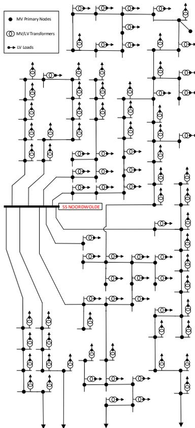
Figure 3. Simulation test NW distribution network.
