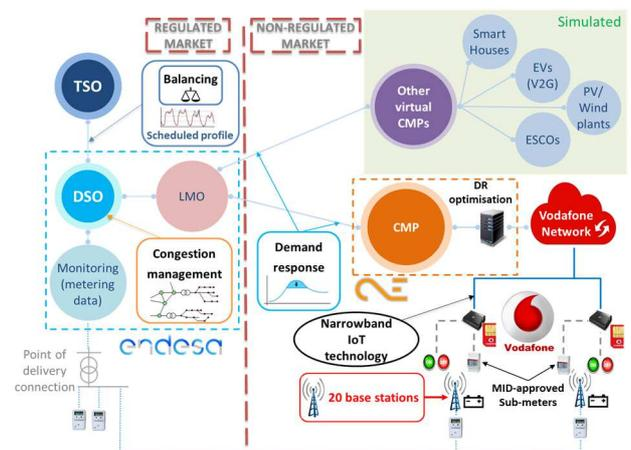
Figure 1. General architecture of the pilot project
