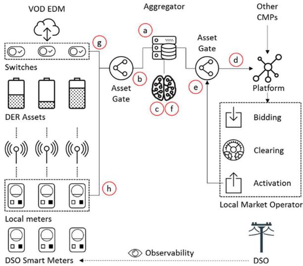
Figure 3. Process flow to create the flexibility bids
