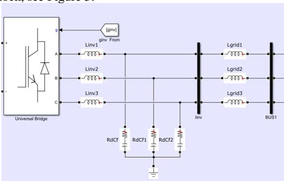
Figure 5 - Three-phase inverter and filter model
