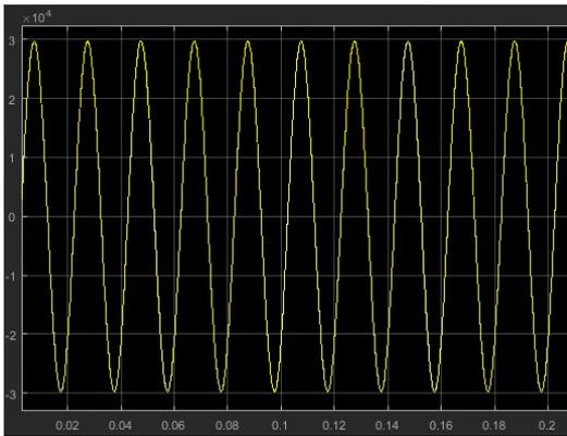
Figure 9 - Voltage profile at train 6 pantograph (High train numbers with 40 EV's charging)
