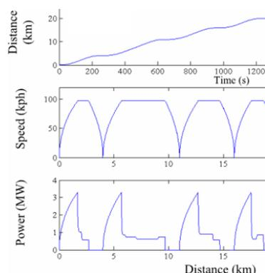
Figure 2 - Class 319/390 Speed and Power Profiles[12]
