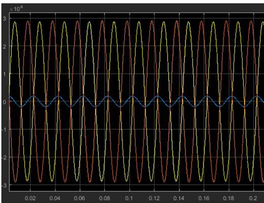
Figure 10 - Voltage at furthest auto-transformer (High train numbers with 80 EV's charging)
