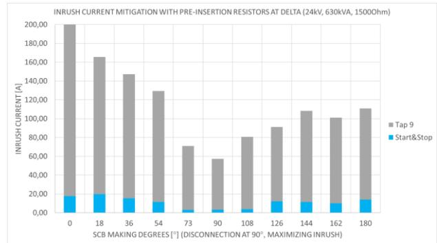
Figure 10. Maximum inrush at Tap 9 vs Start&Stop, with different making degrees and disconnection at 90°.
