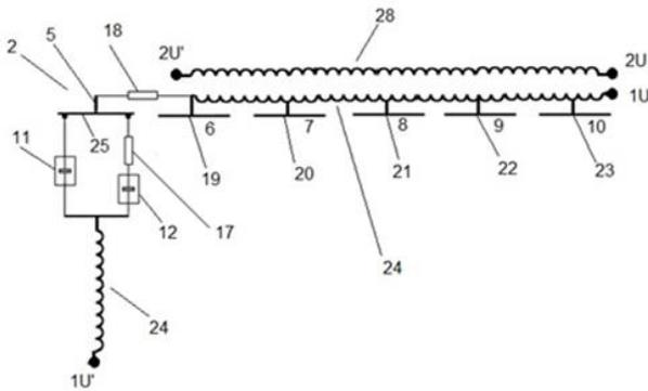
Figure 4. Diagram (from the patent) of the Start&Stop configuration of the OLTC (18. PIR)
