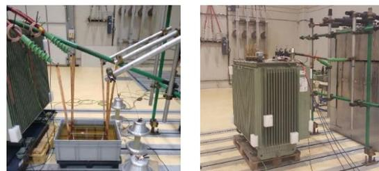
Figure 7. Smart Transformer with PIR in series with lines (left) and inside the transformer (right).
