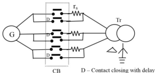
Figure 1. Resistance connected in series to lines with 2 auxiliary contacts per phase [13].
