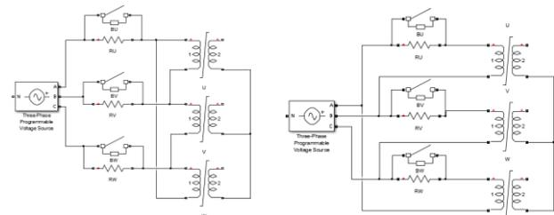
Figure 6. PIR simulation in series with lines (left) and within the delta connection (right).
