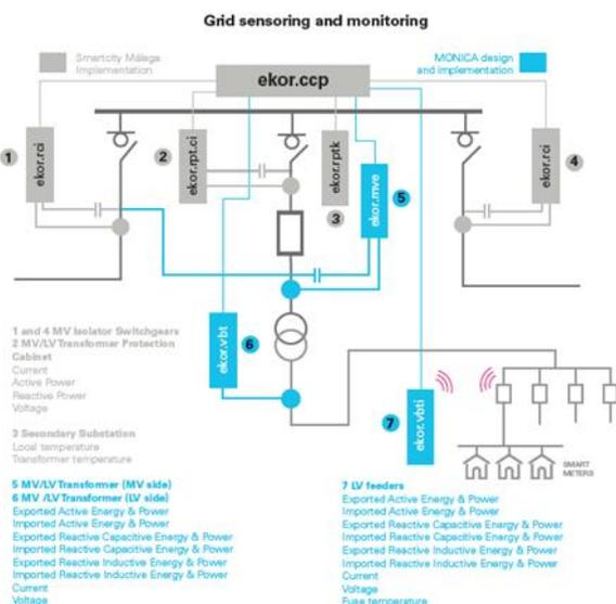
Figure 1. Sensorized Secondary Substation schema.
