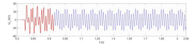
**Figure 6.** Selected first 10 periods of line-to-ground voltage  $U_{fl}$  analyzed by FFT
