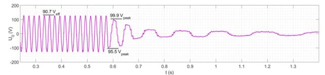
**Figure 13.** Waveform of open delta voltage
