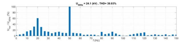
**Figure 7.** The FFT result for the first 10 periods of line-to-ground voltage  $U_{fl}$
