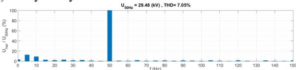
**Figure 17.** The FFT result for the selected 10 periods of line-to-ground voltage  $U_{l1}$
