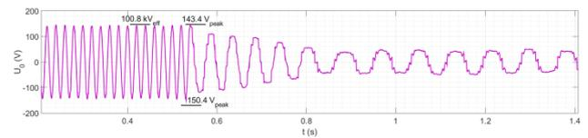
**Figure 5.** Waveform of an open delta voltage
