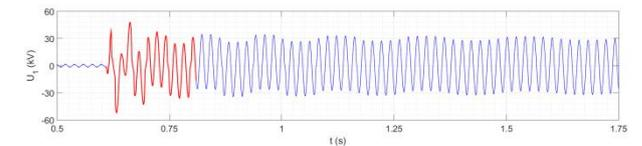
**Figure 14.** Selected first 10 periods of line-to-ground voltage  $U_{J1}$  analyzed by FFT
