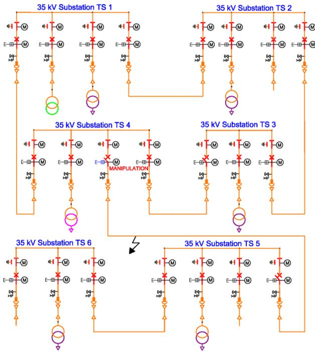
**Figure 2.** The scheme of the test circuit with marked manipulation circuit breaker and earth fault location [8]
