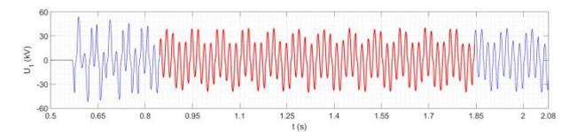
**Figure 8.** Selected 50 periods of line-to-ground voltage  $U_{fl}$  analyzed by FFT
