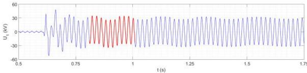
**Figure 16.** Selected 10 periods of line-to-ground voltage  $U_{l1}$  analyzed by FFT
