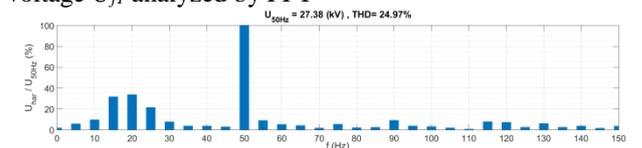
**Figure 15.** The FFT result for the first 10 periods of line-to-ground voltage  $U_{J1}$
