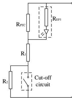
**Figure 10.** Simplified scheme of the VT Guard Pro device [8, 11]
