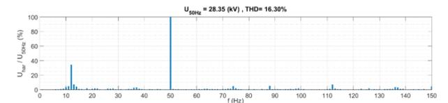
**Figure 9.** The FFT result for the selected 50 periods of line-to-ground voltage  $U_{fl}$
