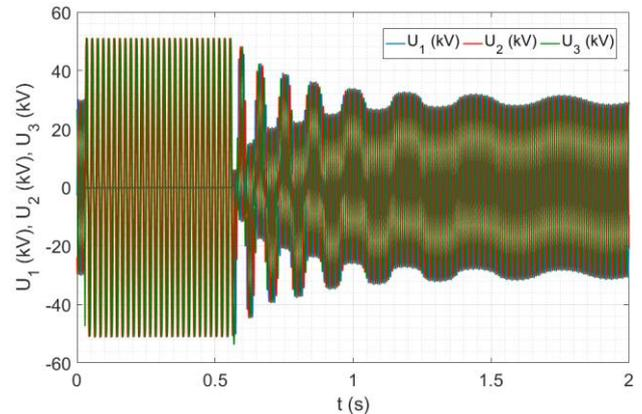
**Figure 12.** Waveform of the line-to-ground voltages
