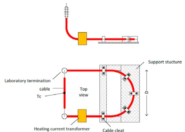
**Figure 3:** Test loop for the overbending test.
