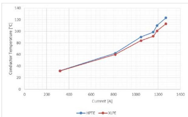
**Figure 2:** Temperature as a function of current.
