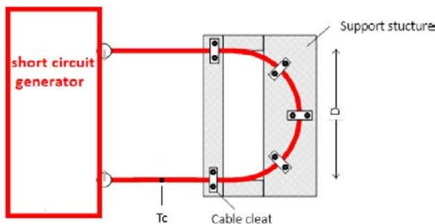
**Figure 4:** Test loop for the short-circuit test.
