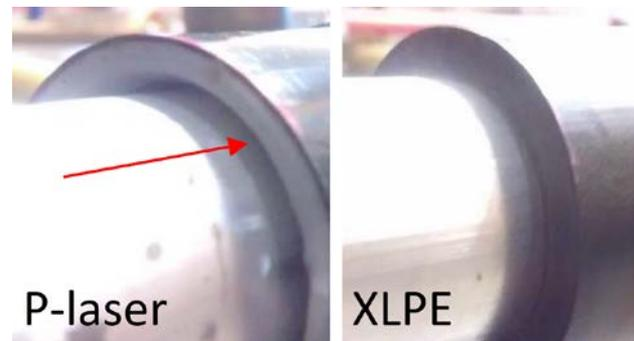
**Figure 5:** Observed shrink behaviour at 50kA/2.25s.
