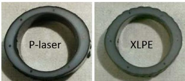
**Figure 6:** Example of distorted shape at P-laser and XLPE after the 50 kA/2.25s short-circuit test.
