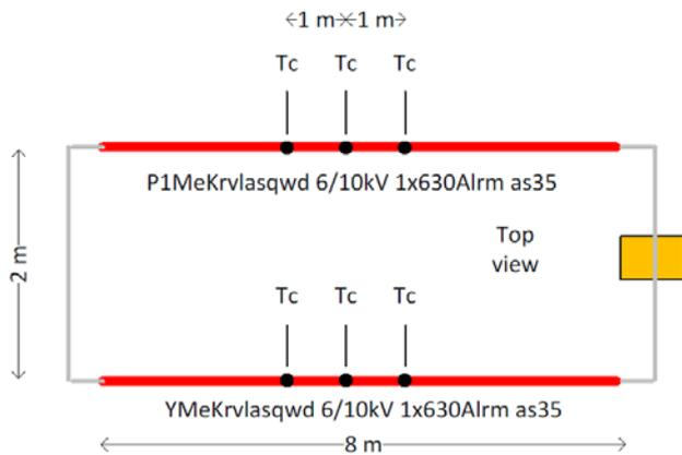
**Figure 1:** Test loop for the ampacity test.
