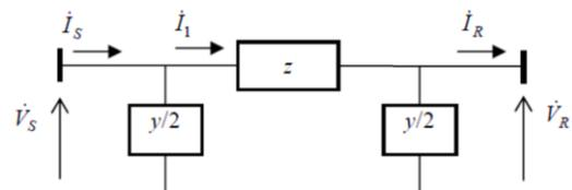
Figure 3 – The  $\pi$ -nominal midline model for one of the phases
