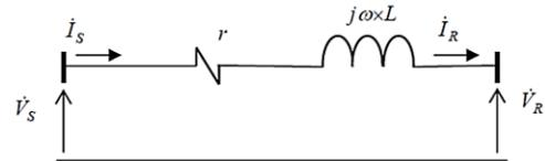
Figure 2 - Short line model for one of the phases
