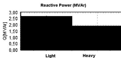
Figure 5 - REACTIVE power calculated without considering the effect of the capacitive reactive of the cables
