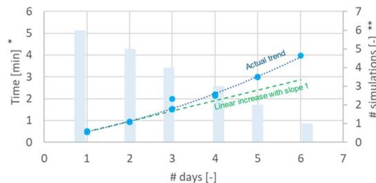
Figure 7: Performance in function of number of days simulated (\*Left-hand y-axis: Simulation time → dots, \*\*Right-hand y-axis: number of simulations → bar diagrams).
