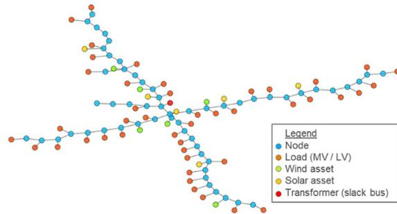
Figure 1: Analysed limited MV network (57 nodes).
