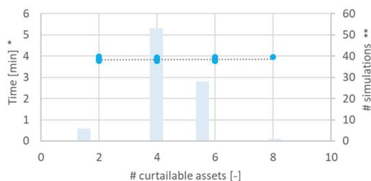
Figure 6: Performance in function of number of curtailable assets (\*Left-hand y-axis: Simulation time → dots, \*\*Right-hand y-axis: number of simulations → bar diagrams).
