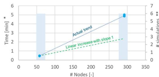
Figure 8: Performance in function of number of nodes simulated (\*Left-hand y-axis: Simulation time → dots, \*\*Right-hand y-axis: number of simulations → bar diagrams).
