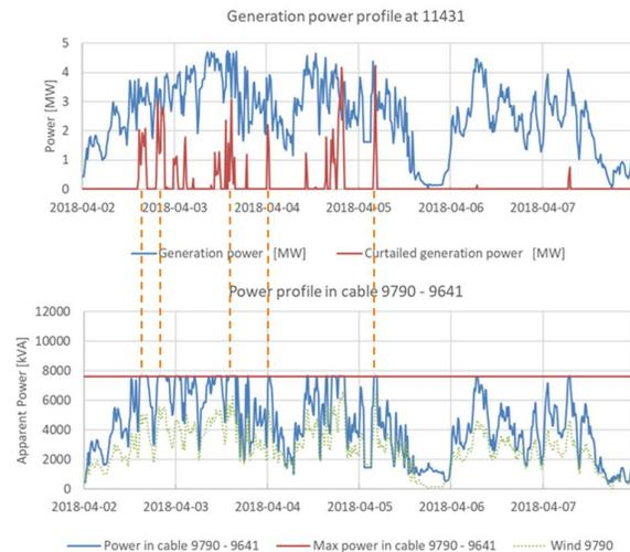
Figure 4: Example of grid congestion management (i.e. power capacity limit) through optimal flexibility activation: wind farm curtailment to respect power capacity limit in the MV cable #9790-9641.
