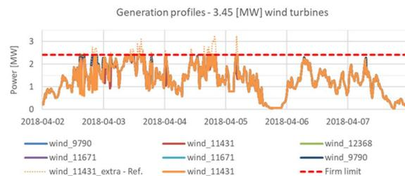
Figure 5: Obtained wind turbines generation profiles after imposing firm limit (i.e. 70% of 3.45 MW installed capacity) vs. reference generation profile (i.e. orange dotted line).
