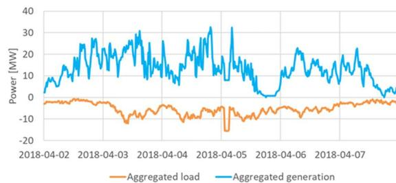
Figure 3: Aggregated load (LV/MV) & generation (Wind & Solar assets) profiles of the limited MV network over 6 days in April.
