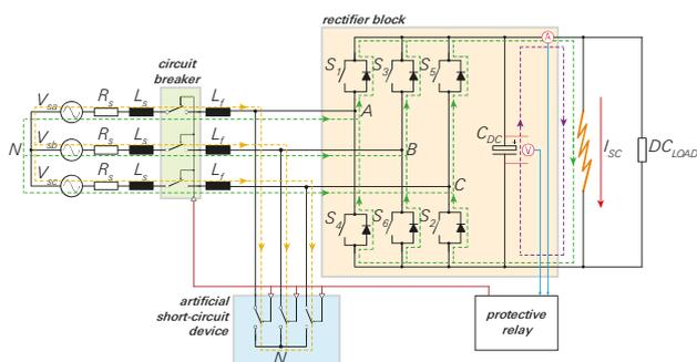
Fig. 8. Schematic diagram of artificial short-circuit method.
