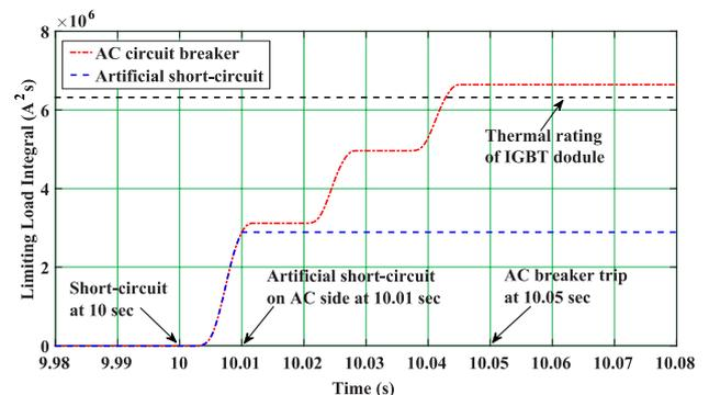
(b) short-circuit energies for the two protection methods
