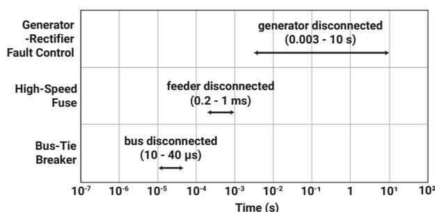
Fig. 3: Time frames of three-level protection method.
