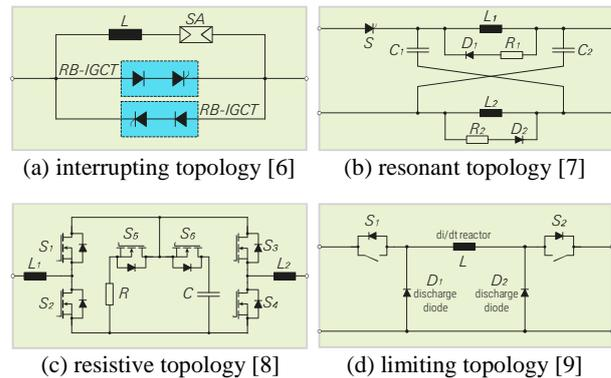
Fig. 4. Solid-state bus-tie breakers for DC distribution systems.
