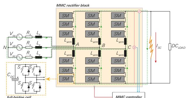
Fig. 10. Schematic diagram of DC short-circuit in MMC.
