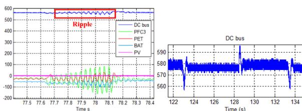
Figure 11: DC voltage ripple
