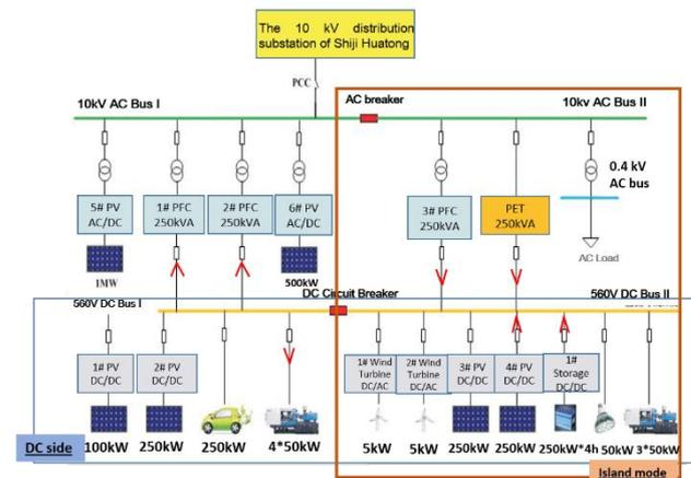
Figure 1: Shangyu AC/DC hybrid microgrid configuration
