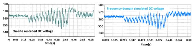
Figure 14: (a) on-site recorded DC voltage; (b) frequency domain simulated DC voltage
