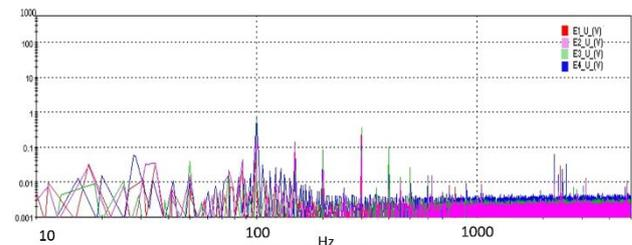
Figure 12: harmonics spectrum for DC bus voltage
