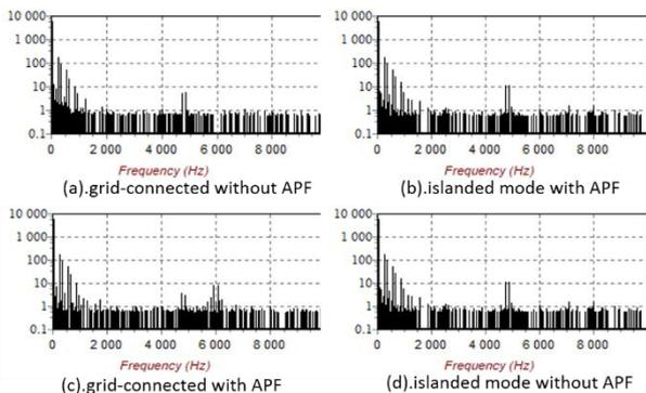
Figure 10: harmonics spectrum for AC bus voltage
