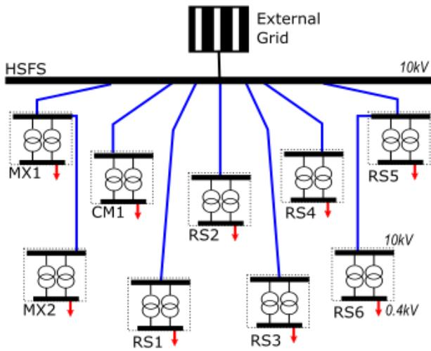
Figure 1 Single line diagram of the 10kV/0.4kV network.
