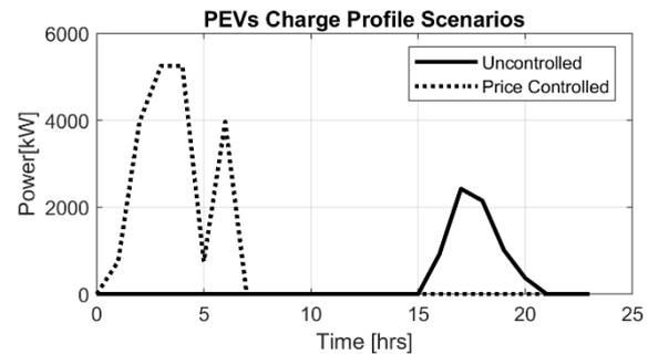
Figure 6 Uncontrolled and price controlled PEV charging profiles
