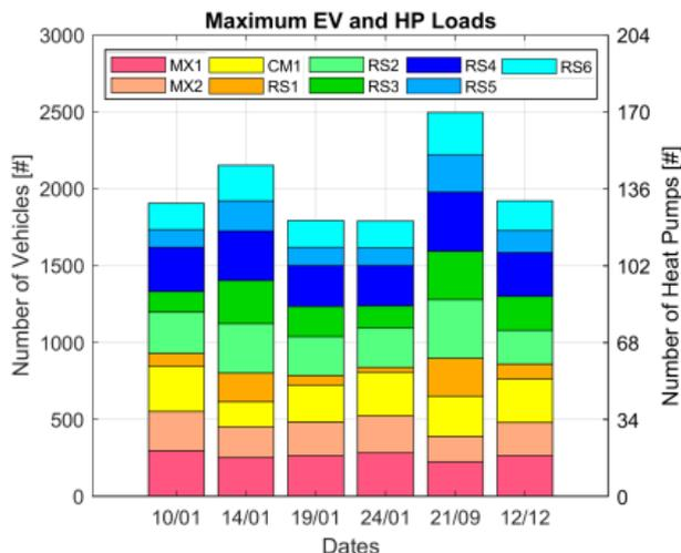
Figure 3 Maximum allowance of PEVs and HPs for the uncontrolled loading case.
