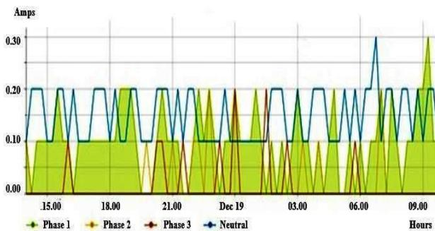
**Fig. 5** The current measured by the sensors installed on CEZ LV OHL
