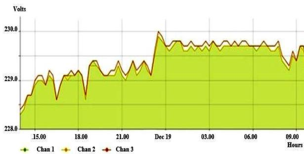
**Fig. 6** The voltage measured by the sensors installed on CEZ LV OHL
