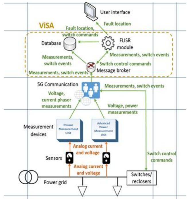
**Fig. 7** Information layer of the FLISR Service developed in SOGNO
