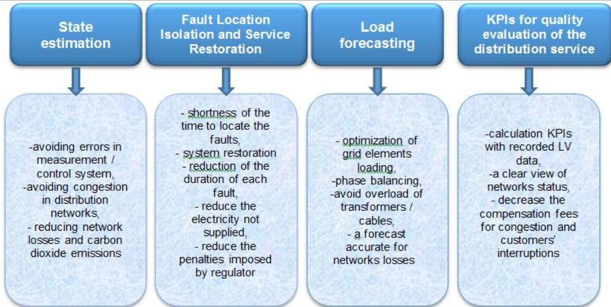
Fig. 3 - Services developed within the SOGNO project
