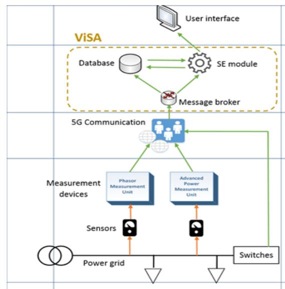
Fig. 4 Component layer of the SE Service developed in SOGNO
