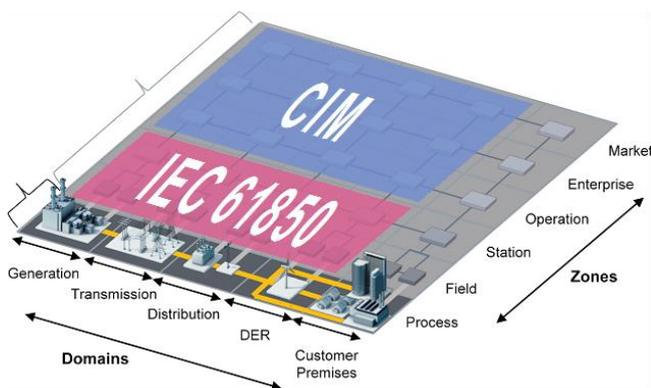
Figure 1: IEC TC57 promotes the use of IEC 61850 standards for process and field implementation and CIM for implementations in higher zones.
