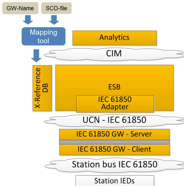
Figure 3: An overview of the IEC 61850 information flow: IED – Gateway – ESB – Analytics application. The SCD file is used for configuration of the relation database.
