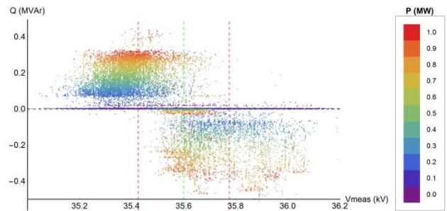
Fig. 11: Long-term statistical assessment of volt-var control system behaviour on PV Zamberk (installed capacity 1.1 MWp)
