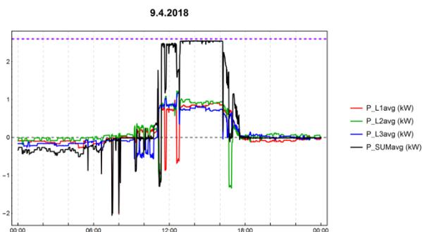
Fig. 12: Daily behaviour of customer with PV and energy storage – PV 5.2 kWp, feed in power limited to 50 % (2.6 kW)
