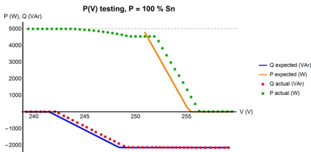
Fig. 6: P (V) function lab test results for Fronius PV inverter
