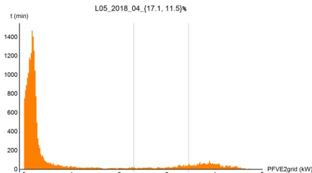
Fig. 14: Net PV production without any energy storage – PV 4.6 kWp
