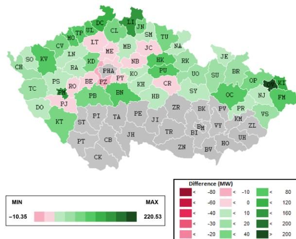
Fig. 15: Expected lack of DER hosting capacity in LV grids in 2040 in case that smart grid solutions are implemented
