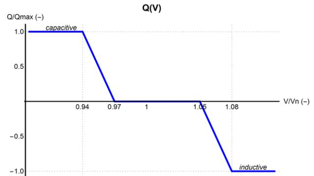
Fig. 3: Autonomous Q (V) function of smart PV inverter
