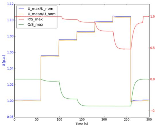
Fig. 7: Control dynamic behaviour for Fronius PV inverter
