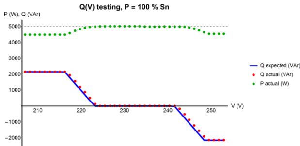
Fig. 5: Q (V) function lab test results for Fronius PV inverter
