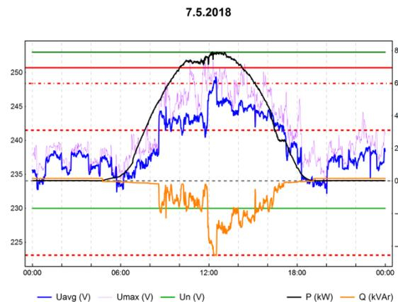
Fig. 8: Daily behaviour of smart PV inverter with Q (V) and P (V) functions
