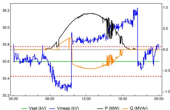
Fig. 10: Demonstration of volt-var control system on 1.1 MWp PV
