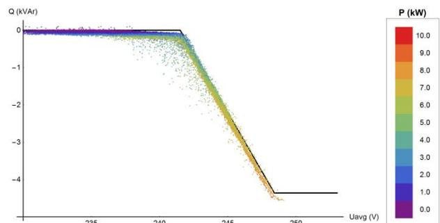
Fig. 9: Smart PV inverter operation points in April 2018
