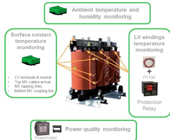
Figure 1 Cast Resin Transformer monitoring [1]
