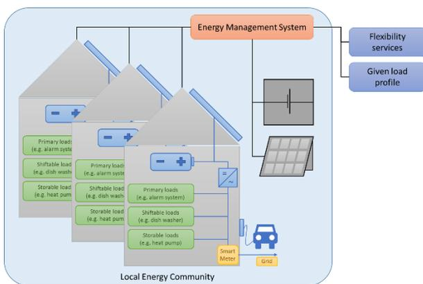
Figure 3: Model of a local energy community with different households, community storage, and PV, providing flexibility services and following a given load profile.
