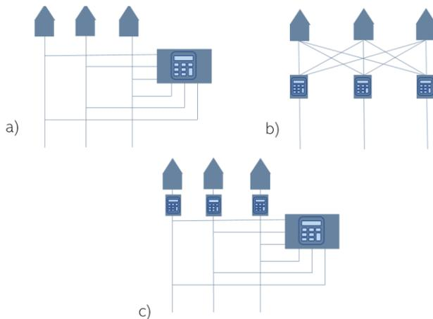
Figure 6 Different architectures for realizing a common EMS: a) Centralized b) Decentralized (every household has access to all information of the other households, possibly by using a blockchain) c) Mixed (division of tasks in centralized and decentralized ones).
