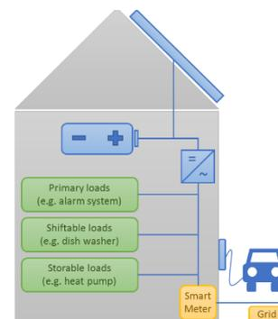
Figure 1: Household with different types of loads (primary, shift-able, storable), PV, battery, inverter, smart meter, electric vehicle, and grid connection
