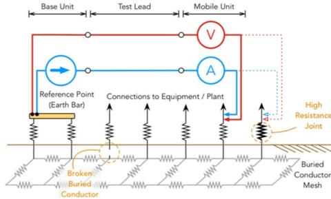
**Figure 5.** Integrity or Continuity Testing Example
