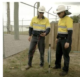
**Image 1.** Earthing System Step Voltage Testing
