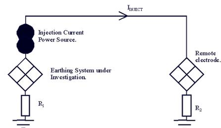
**Figure 4.** Earthing System Impedance Testing
