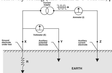
**Figure 3.** Common Grid Resistance Testing
