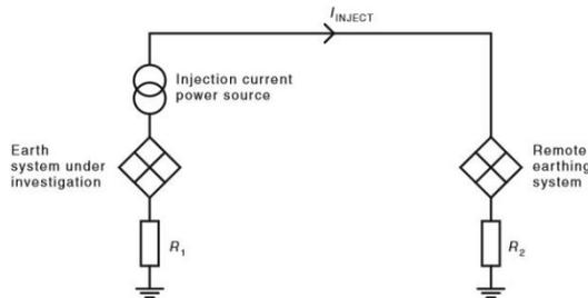
**Figure 1.** The Basic Test Circuit from AS 2067.
