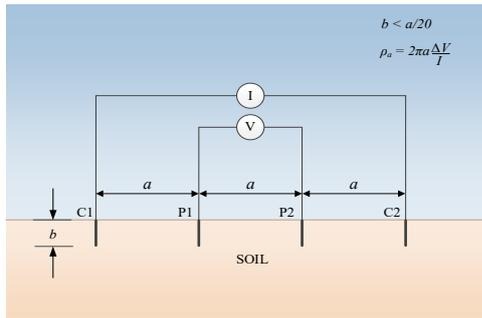
**Figure 2.** Wenner Soil Electrical Resistivity Test Method
