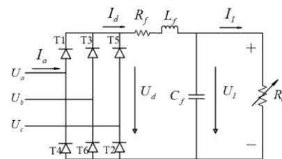
Figure 1 Equivalent model of EV charger
