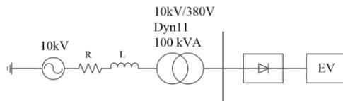
Figure 3 A typical example of low voltage distribution network
