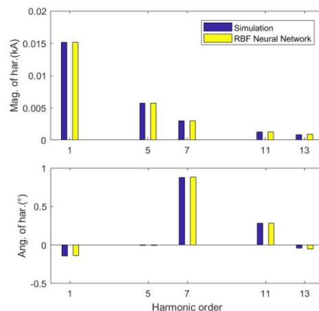
Figure4 Comparison of the model output results
