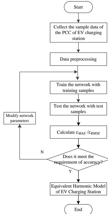
Figure 2 Harmonic Modeling Process of EV Charging Station Based on RBFN
