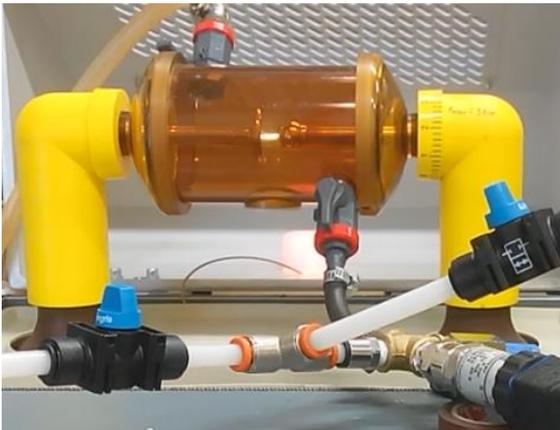
Fig 1. Used hermetic cell with the electrodes.
