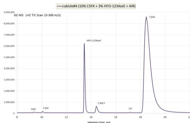
Fig. 4 GC-MS chromatogram of gas sample extracted.
