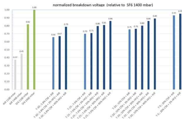
Fig 2. Comparison of breakdown voltage for different mixtures
