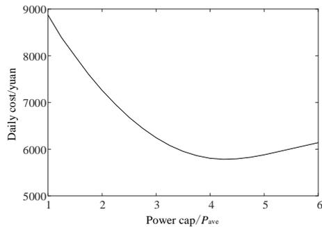
Fig. 6 The impact of power cap of grid on daily cost
