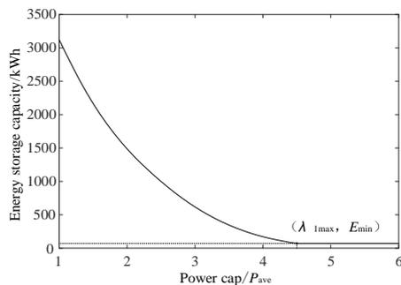
Fig. 7 The impact of power cap of grid on ESS capacity
