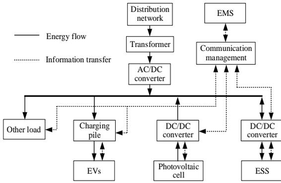
Fig. 1 Structure of PV integrated EV charging station
