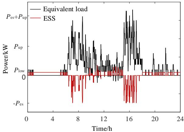
Fig. 2 Power curve of equivalent load and ESS
