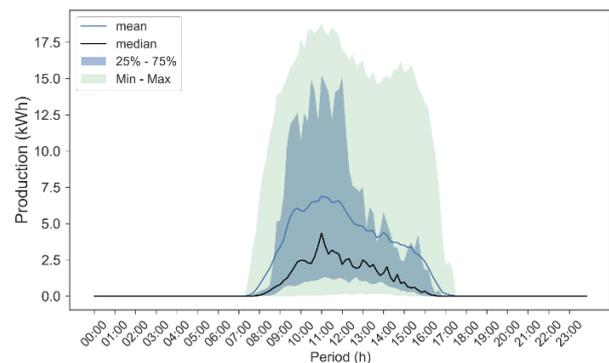
**Figure 2.** Solar production from the service building in February 2017 [9].
