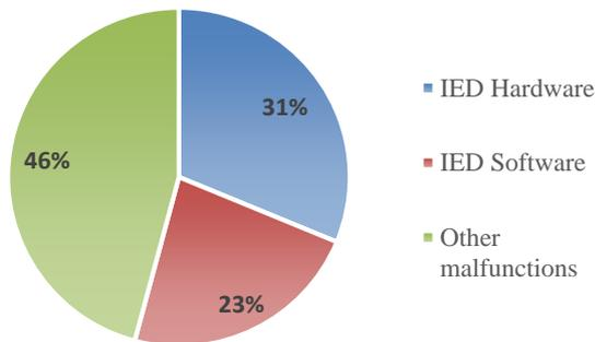
Figure 2 - Detected malfunctions during TBM (data from 38 installations during 2018)
