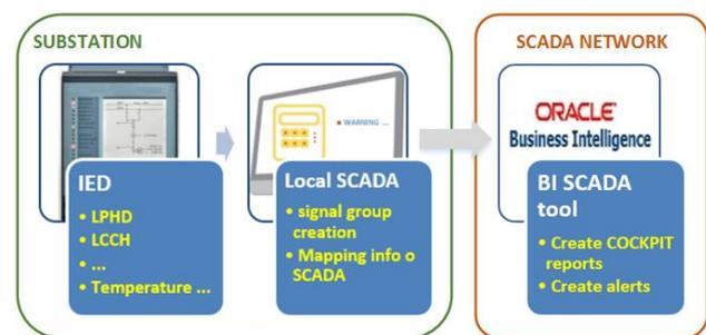
Figure 6 – IEC 61850 IED self-monitoring information mapping and reporting architecture
