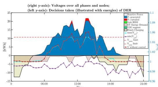
Figure 4 Extreme voltages over all phases and nodes; DER state along 24-hours for scenario C3a.
