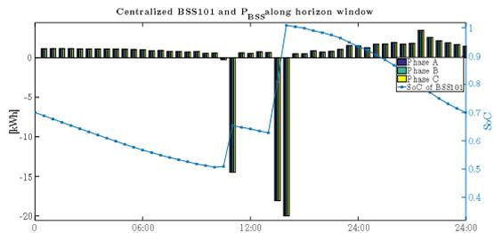
Figure 3 Control setpoints for BESS101 at scenario C1b, for the 24-h.
