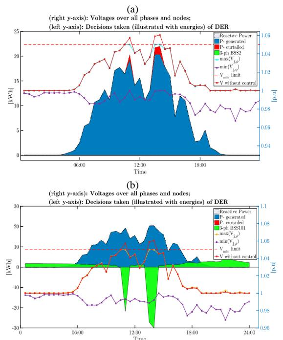
Figure 2 Extreme voltages over all phases and nodes; DER state along 24-hours for scenario (a) C1a and (b) C1b.
