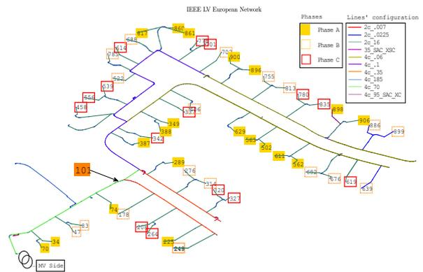
**Figure 1** IEEE Low Voltage grid test case.
