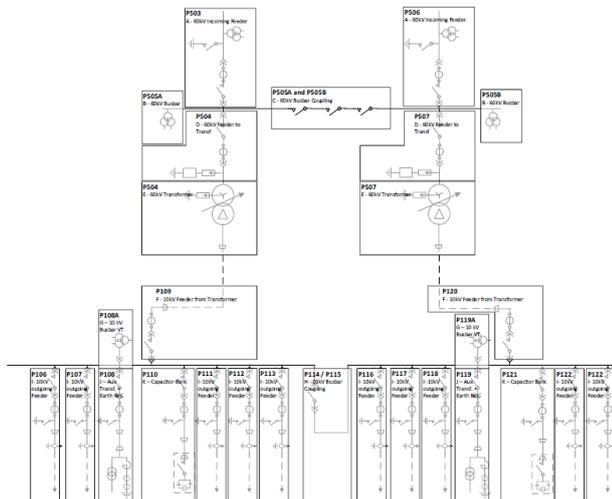
Figure 4. Substation electrical scheme.
