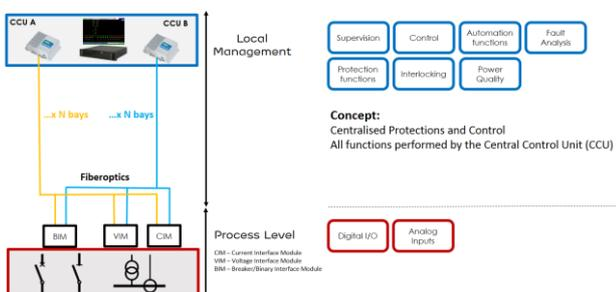
Figure 3. EGDE Digital Substation SAS System Architecture.
