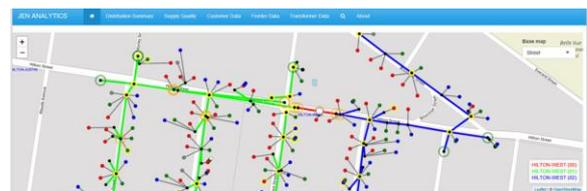
Fig.4. Visualization of a LV network with customer phase colouring
