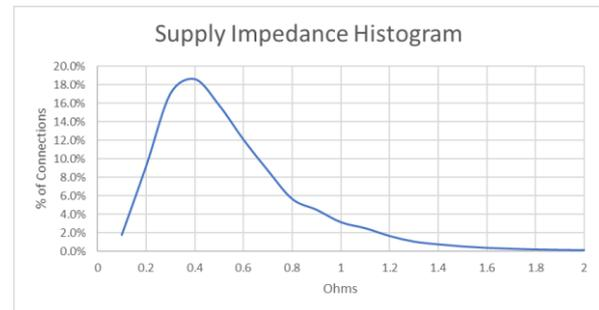
Fig.8. Variation of supply impedances for Jemena’s 335,000 AMI meters
