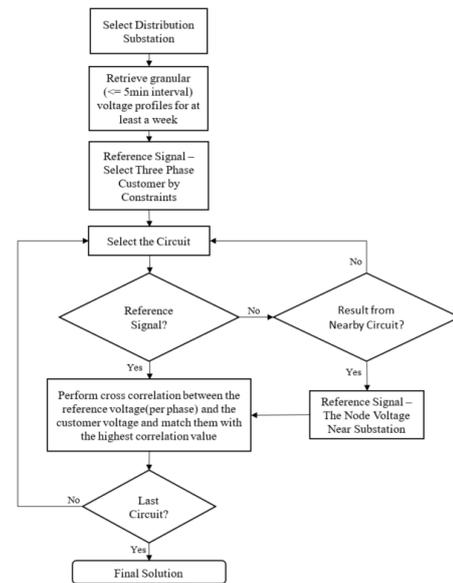
Fig.3. Flow chart of phase identification based on cross correlation
