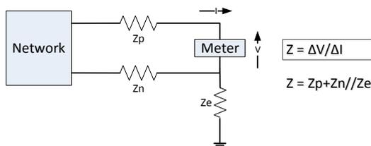
Fig.7. Principle of supply impedance measurement
