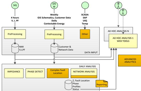
Fig.2. High level architectural diagram of the Jemena data analytics setup
