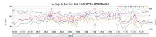
Fig.5. Estimated voltages and currents at a 22kV/415V distribution substation
