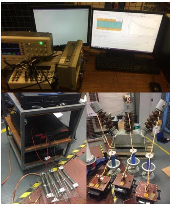
Figure 1 – Laboratory setup; top: LabVIEW DAQ and oscilloscopes; bottom left: audio amplifiers; bottom right: 30 kV test transformers, voltage dividers, and example test object (33 kV 3-phase VT)
