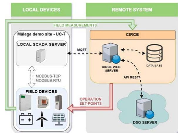
Fig. 1. Global operation schema of the solution.
