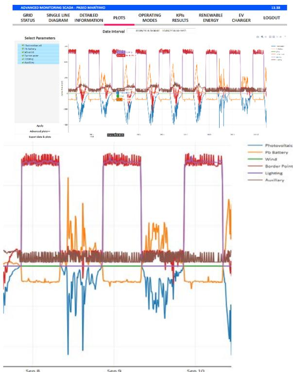
Fig. 5. SCADA showing the operation of the microgrid operation (general view and detail).
