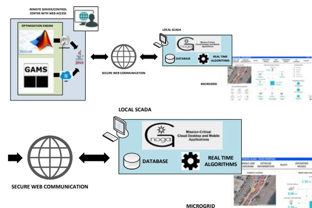
Fig. 2. Local SCADA system in the global communications schema.
