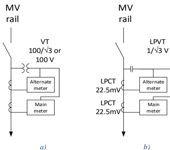
Figure 1a: A single line diagram of a typical revenue metering setup for connections with contracted power larger than 1 MW.
