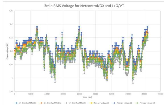
Figure 3: Voltage measurements (3 minutes RMS average) during one day period.
