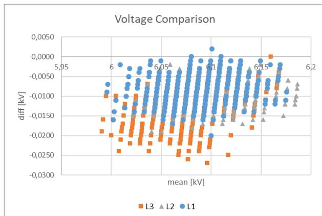
Figure 5: Mean versus difference plot for the voltage measurements of phase L1, L2 and L3, during one day.
