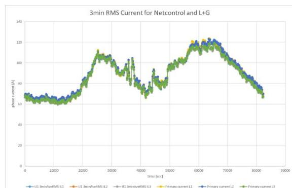
Figure 4: Current measurements (3 minutes RMS average) during one day period.
