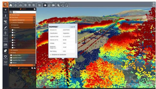
**Figure 9.** Example of Intrusion point locations within 4 metres from the conductor on 33kV circuit with point cloud coloured by height in Roames World. The defect in the foreground is 3.55m from the conductor. The Intrusion Clearances Layer menu is open on the left.
