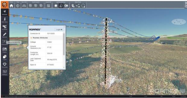
**Figure 6.** Roames World point cloud of 132kV tower on a European operators network
