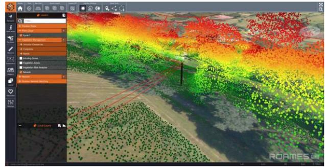
**Figure 8.** Roames World Visualisation of vegetation shape around power lines using the point cloud data
