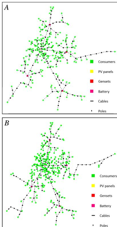
Figure 2: Optimal mini-grid in scenario 1 (A) & 2 (B)
