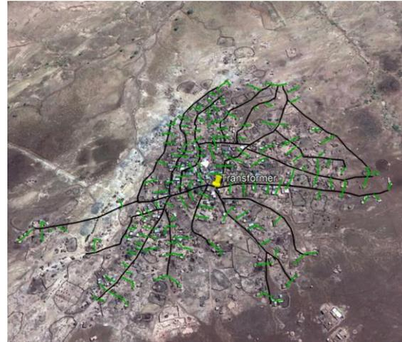
Figure 1: Aerial view of Kokoloko village with an LV network traced manually
