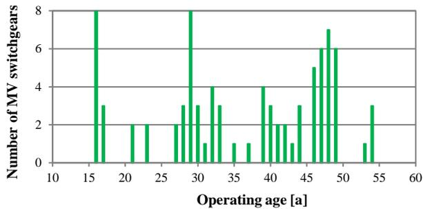
**Figure 7** Distribution of the age structure of the MV switchgears tested in the laboratory
