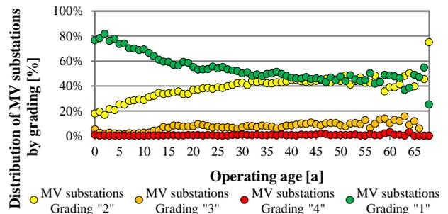
**Figure 5** Percentage distribution of the MV substations by grading
