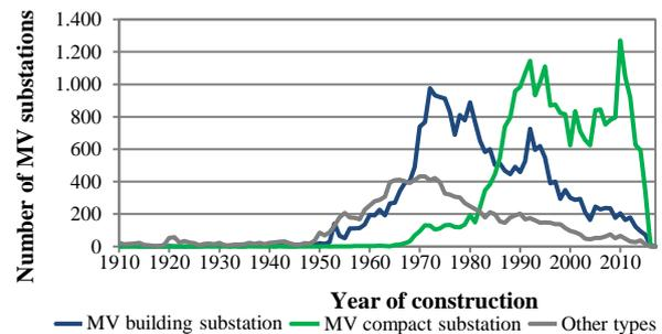
**Figure 1** Distribution of the number of different types of MV substations for the different years of construction
