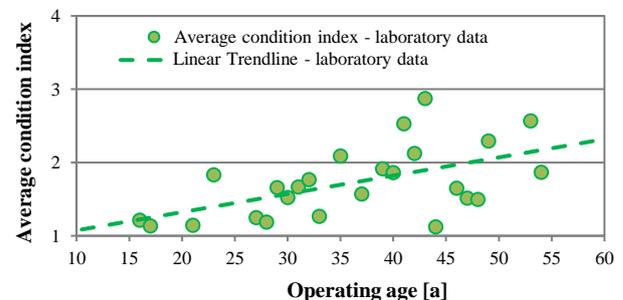
**Figure 9** Ageing behaviour of the tested MV switchgears
