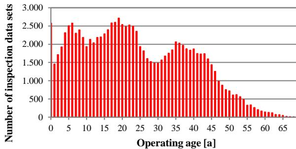
**Figure 3** Distribution of the age structure of the MV substations of all eleven DSOs
