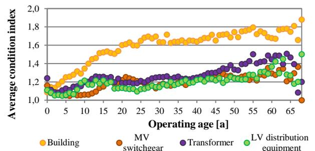
**Figure 6** Ageing behaviour of the main components of the MV substations based on the inspection data
