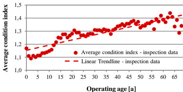
**Figure 4** Ageing behaviour of the MV substations based on the inspection data
