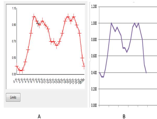
Figure 4 – Residential load profile representation in A) DIgSILENT B) MS EXCEL – Data from [5-6]
