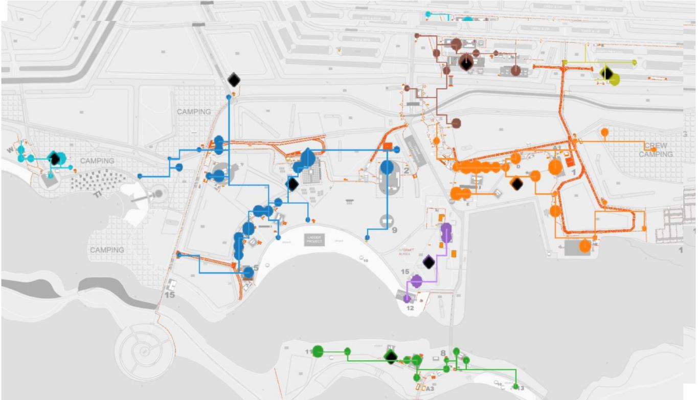
The AI output results in somewhat higher power, compared to the human designs, mainly due to the redundancy factor applied, as well achieving a saving on the grid length. For both festivals, the savings on grid length exceed 40% compared to the realised planning (see table 2 and 3). The cost savings versus the realized plans is around 30%.
