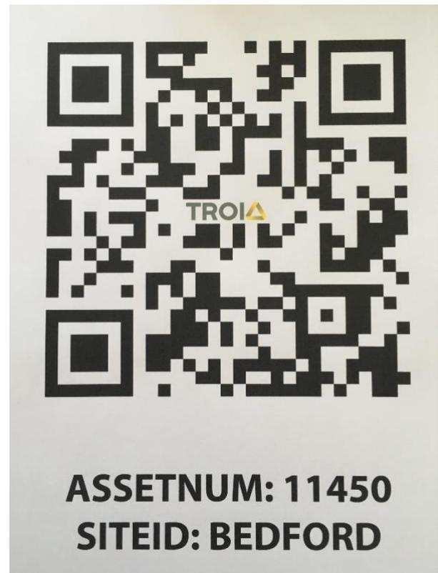
Picture 9 QR code placed on Asset and links ASSETNUM from IBM Maximo.
