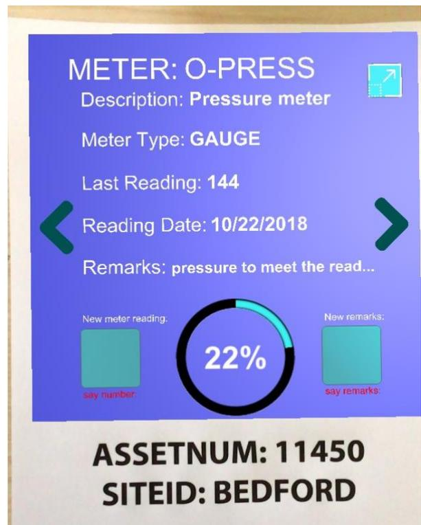
Picture 10 AR info real-time content about asset sensors displayed over QR code.
