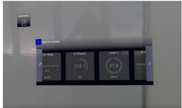
Picture 4 Review of the SCADA / IoT readings on the glasses.
