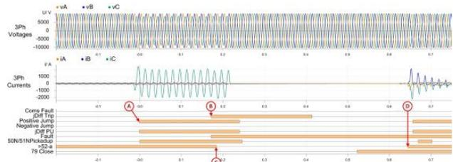
Figure 9 - COMTRADE Fault record from controller device
