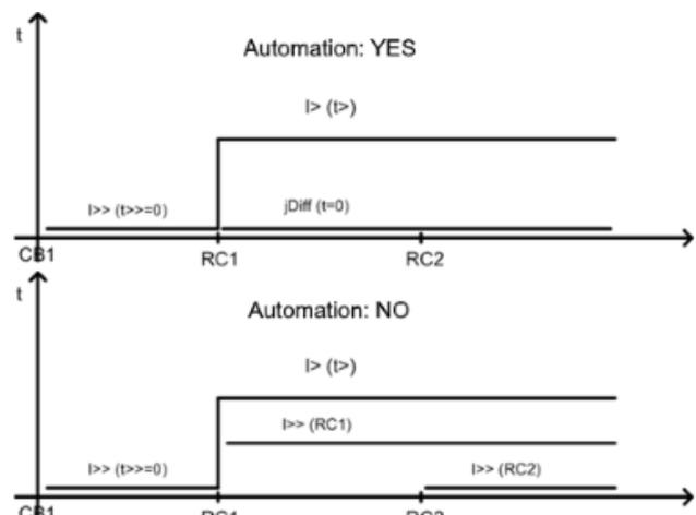
Figure 7. Protection coordination in zone 1 with and without communication (automation)
