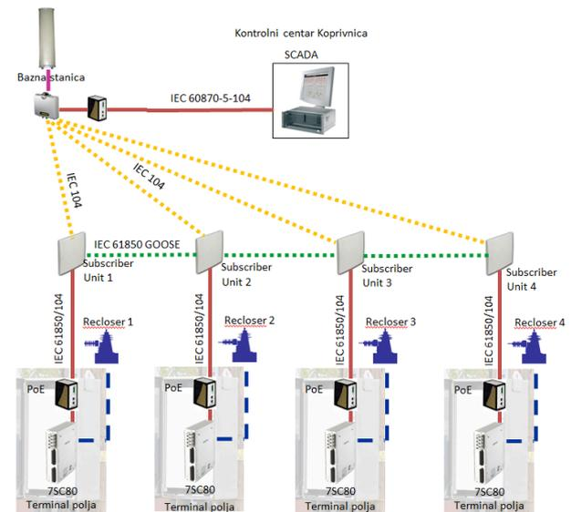
Figure 2 - Schematic diagram of selfhealing grid Koprivnica
