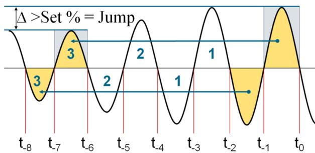
Figure 5 - Jump Differential detector
