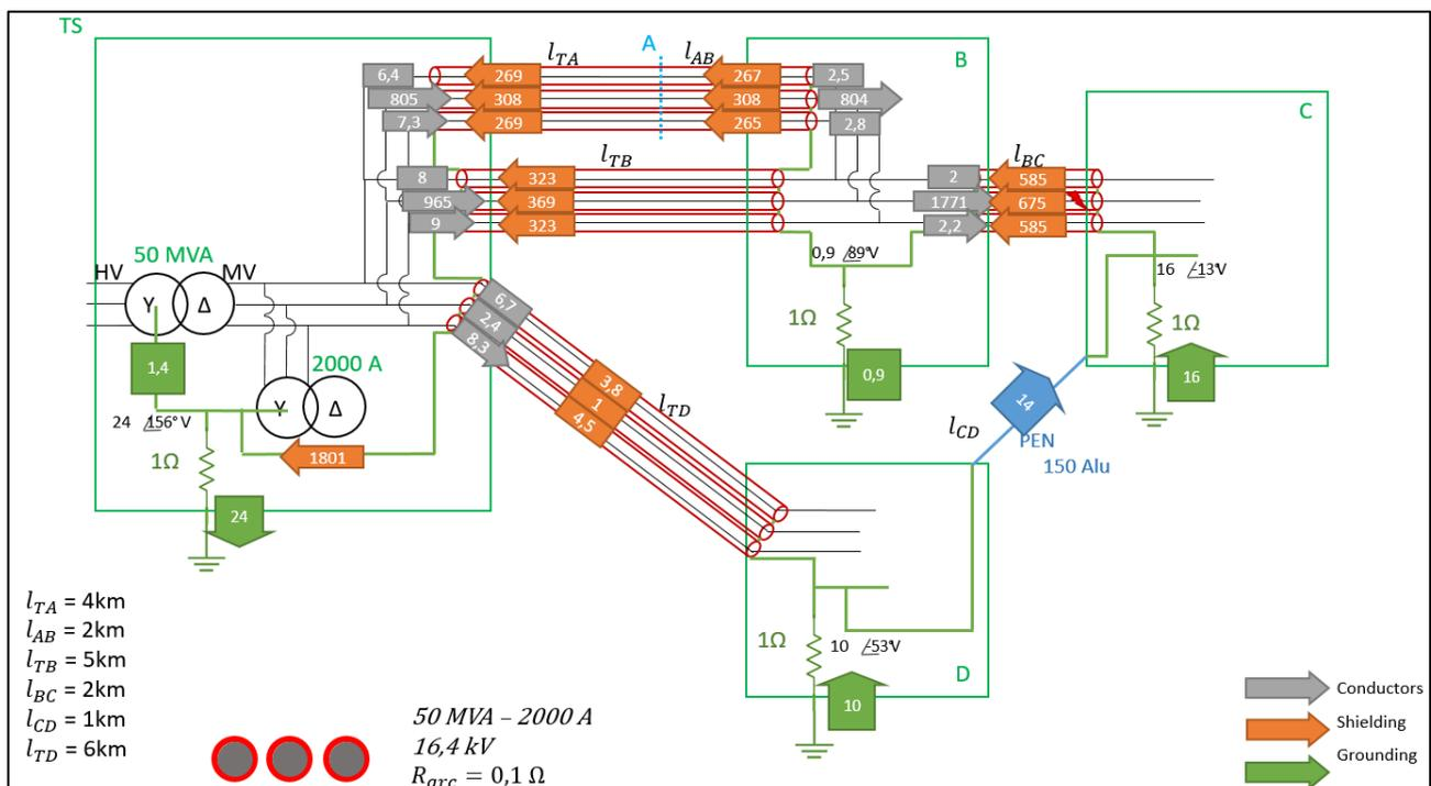
Figure 5: Results of a fault simulation close to substation C in the modelled circuit
