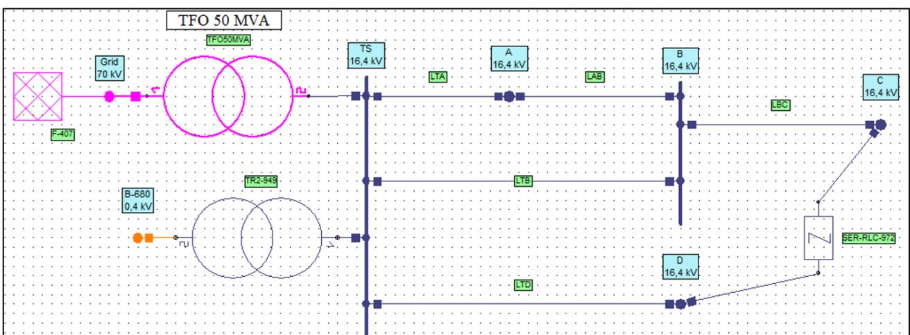
Figure 7: NEPLAN® model of the first MV network studied
