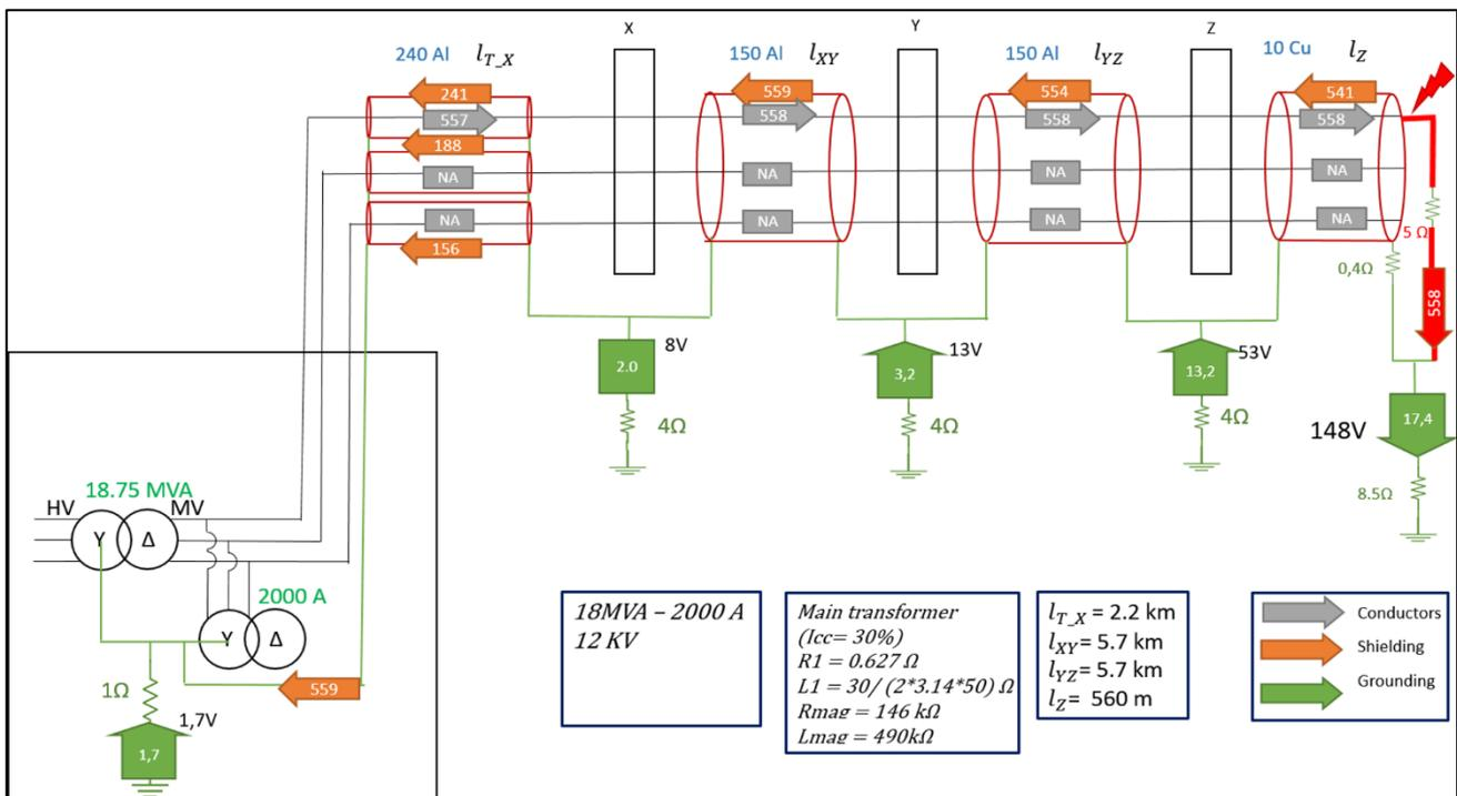
Figure 6: Results of a fault on another circuit modelled
