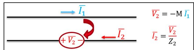
Figure 1: Lenz law applied to two adjacent conductors
