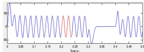
Fig. 6 (b) stator current without STATCOM
