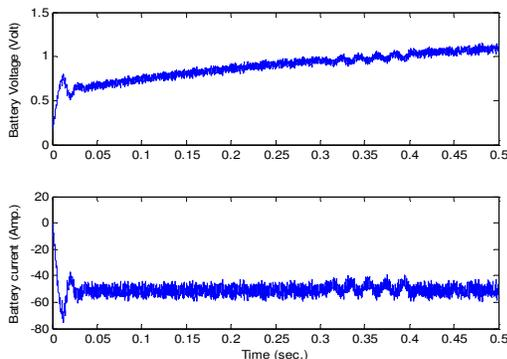
Fig. 19, Battery voltage and current
