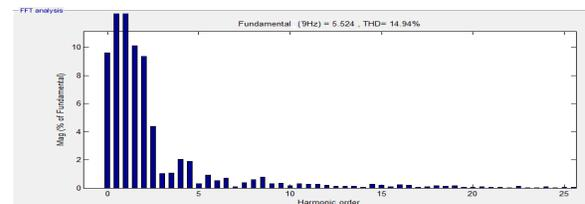
Fig. 14, THD of rotor current during grid fault
