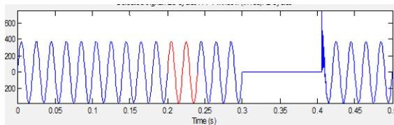
Fig. 3 (b) Stator voltage without STATCOM
