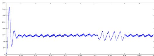
Fig. 16 (a) Electromagnetic Torque with STATCOM
