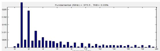
Fig. 4, THD of stator voltage during normal operation
