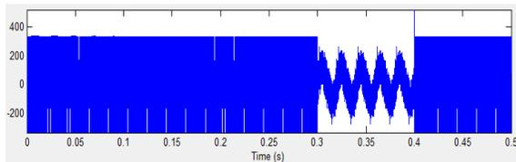
Fig. 3 (a) Stator voltage with STATCOM
