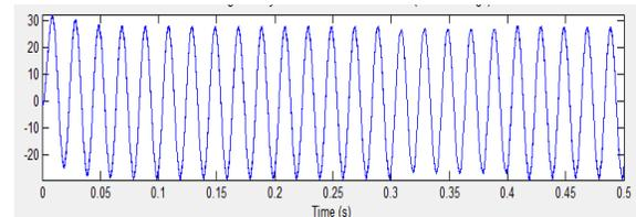
Fig. 6 (a) stator current with STATCOM
