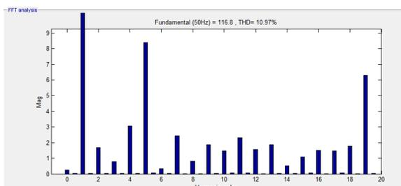
Fig. 5, THD of stator voltage with STATCOM during grid fault
