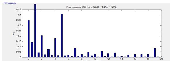
Fig. 8, THD of stator current with STATCOM during grid fault
