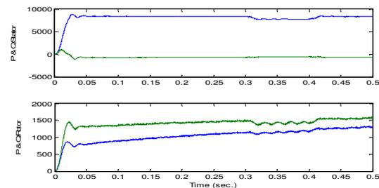
Fig. 15 (a) active &amp; reactive power of stator &amp; rotor with STATCOM
