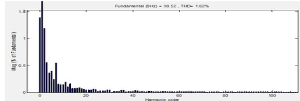
Fig. 13, The THD of rotor current during normal operation
