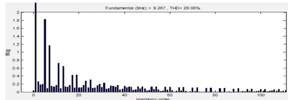
Fig. 10, THD of rotor voltage during normal operation
