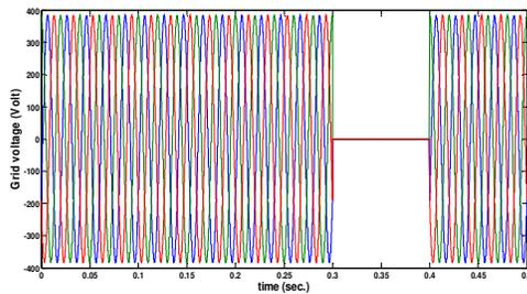
Fig. 2, Grid voltage with ground fault
