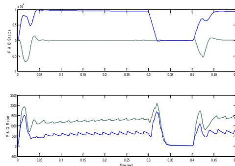
Fig. 15 (b) active &amp; reactive power of stator &amp; rotor without STATCOM.
