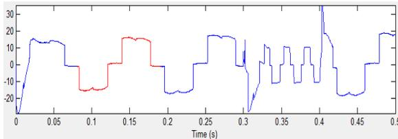
Fig. 9 (b) Rotor voltage without STATCOM
