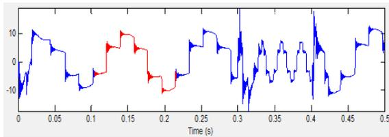
Fig. 9 (a) Rotor voltage with STATCOM
