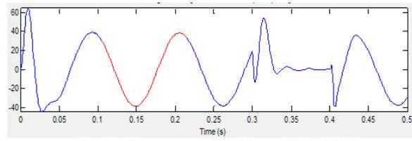
Fig. 12 (b) rotor current without STATCOM
