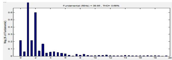
Fig. 7, THDs of stator current during normal operation
