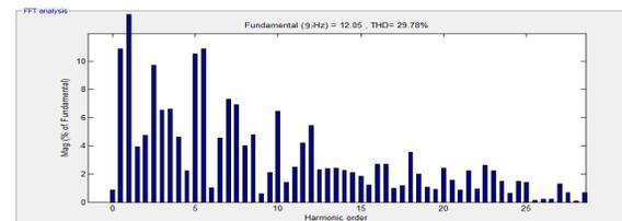
Fig. 11, THD of rotor voltage with STATCOM during grid fault
