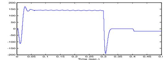
Fig. 18 (b) Electromagnetic Torque without STATCOM
