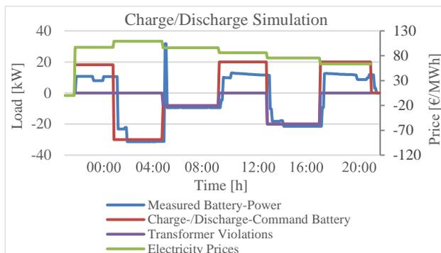
Figure 3 - Real charging and discharging of the VRFB according to load and price signals.
