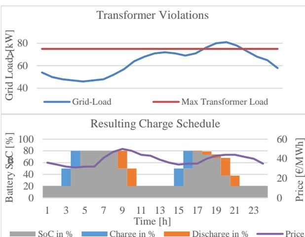
Figure 1 – A: An example load curve and the maximum load of the transformer; B: The charging and discharging schedule resulting from both the load and electricity prices
