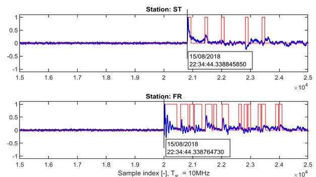
Figure 3: Captured current travelling waves from both side of the line
