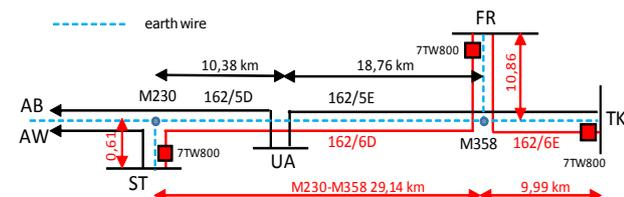
Figure 5: Field installation in a compensated network for the testing of the reliability of the travelling wave technology
