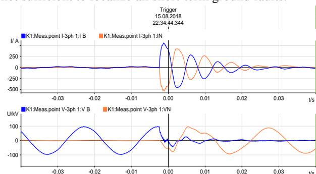
Figure 1: Recorded short-term phase-to-earth fault in a compensated network from figure 5 (Station ST)
