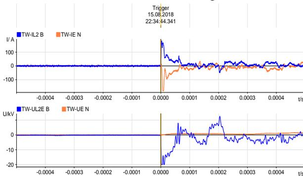
Figure 2: Travelling wave captured by travelling wave fault recorder (Station ST)
