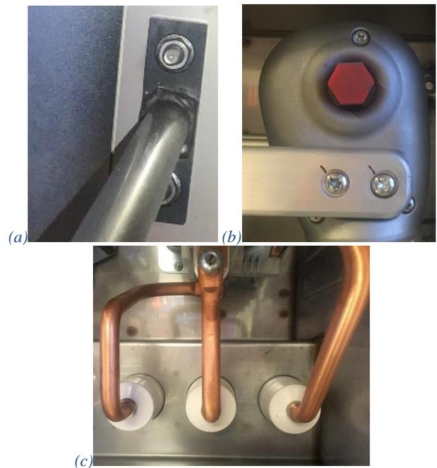
Figure 4. Pictures showing metal components within gas enclosure of field test unit after 3 years of service. (a) Stainless steel internal supporting rod welded to stainless steel plate, (b) cast aluminum vacuum interrupter pole house and extruded aluminum bus bar and (c) bare copper conductors.
