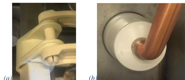
Figure 5. Pictures showing polymer parts from returned and opened field test switchgear. (a) Molded glass fiber filled PBT parts and (b) cast epoxy bushing.
